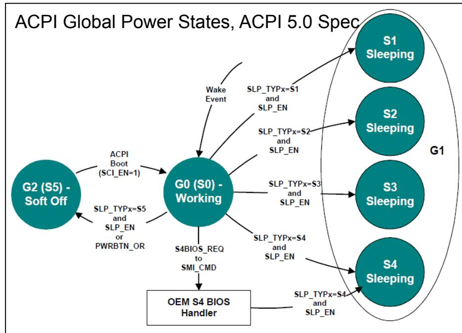
System boot will follow a different path based on what power state its in on startup!
