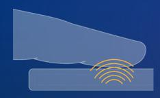
Even stronger ultrasonics penetrate through thicker metal (up to 400  $\mu$ m) and cover glass (up to 400  $\mu$ m), allowing for more design options
